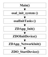
Fig. 4. Equipment general startup process when HOLD\_AUTO\_START is not defined
